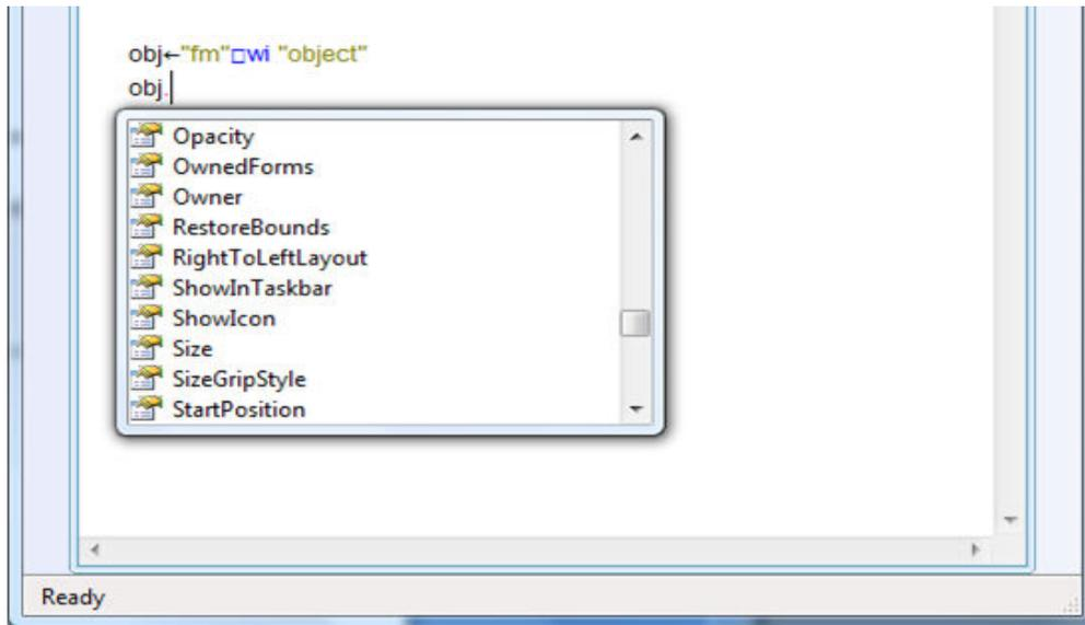
In addition, many new GUI controls are available because all GUI controls supported by the System.Windows.Forms .Net namespace can be accessed by the [wi] feature.
