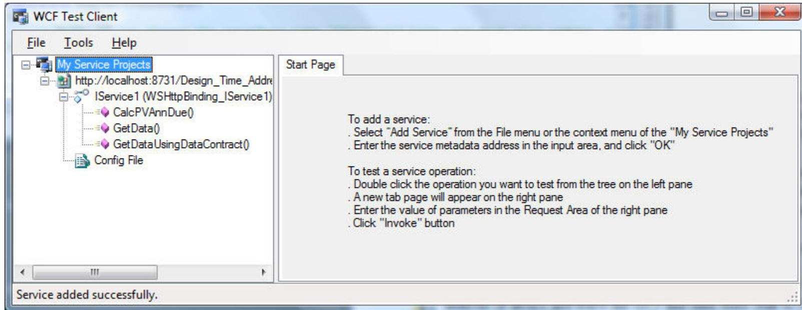
Double click the CalcPVAnnDue() operation on the WCF Test Client surface to test it. Enter reasonable values for the AnnIntPct, years and AnnPmt fields and click the Invoke button to see the result as it would be provided to a web-client which used this web service:
