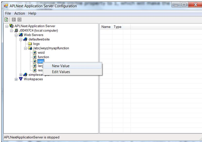
Enter the name of the (1<sup>st</sup>) right argument and select the applicable data type for the right argument. Selecting the applicable data type for a function argument is 'tricky' because it requires knowledge of the client data source and the available web standards [argument data types supported by AAS](#).
